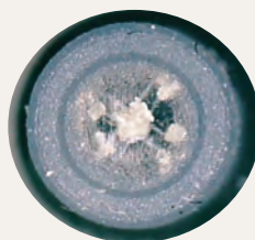
Rain nozzle with QuickClean+, blocked by mineral buildup
